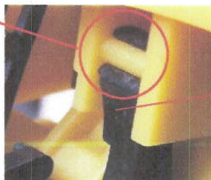
Regulator closer NOT SEATED CORRECTLY
